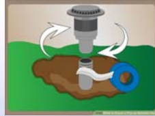
Turning directions on and off Teflon tape helps seal new head
